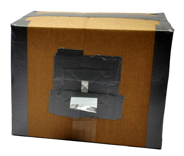
with your duct tape. Do not open the shutter on your pinhole at this stage.
